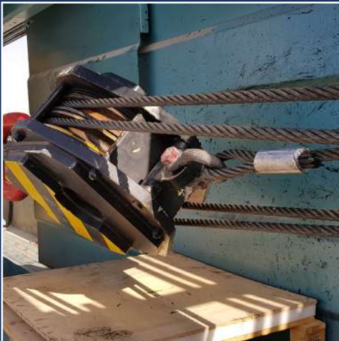
PROOF LOAD TEST OF CRANE HOOK BLOCK
