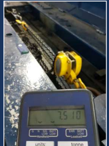
PROOF LOAD TEST OF CHAIN BLOCK
