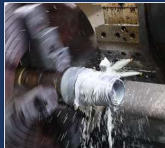
Drill Pipe Connection Threading
