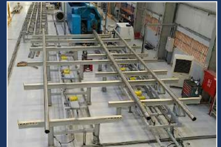
Pipe Handling System
