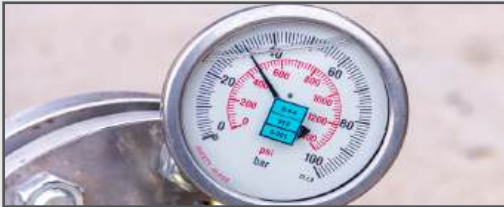
Hydrostatic Pressure Testing
