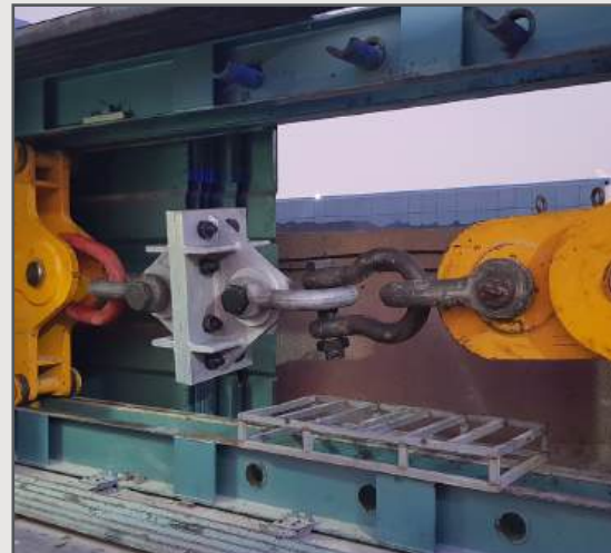
PROOF LOAD TEST OF LIFTING BRACKETS
