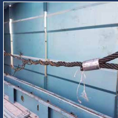
BREAK TEST OF WIRE ROPE SLING
