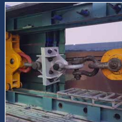
PROOF LOAD TEST OF LIFTING BRACKETS
