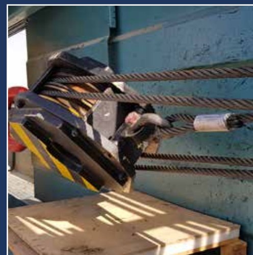
PROOF LOAD TEST OF CRANE HOOK BLOCK
